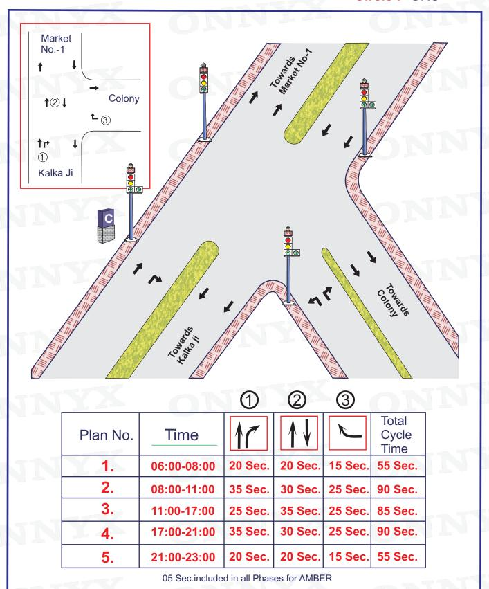
Signal Timing – 06:00 – 23:00 Blinker Timing – 23:00 – 06:00
