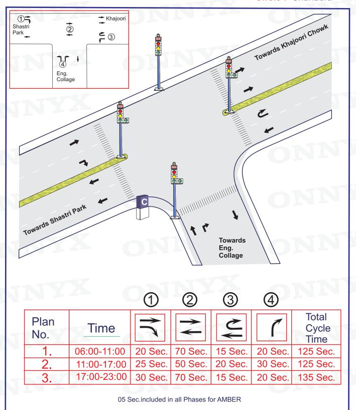
Signal Timing – 06:00 – 23:00 Blinker Timing – 23:00 – 06:00
