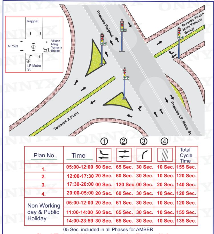
Signal Timing – 24 Hours Blinker Timing – N. A.
