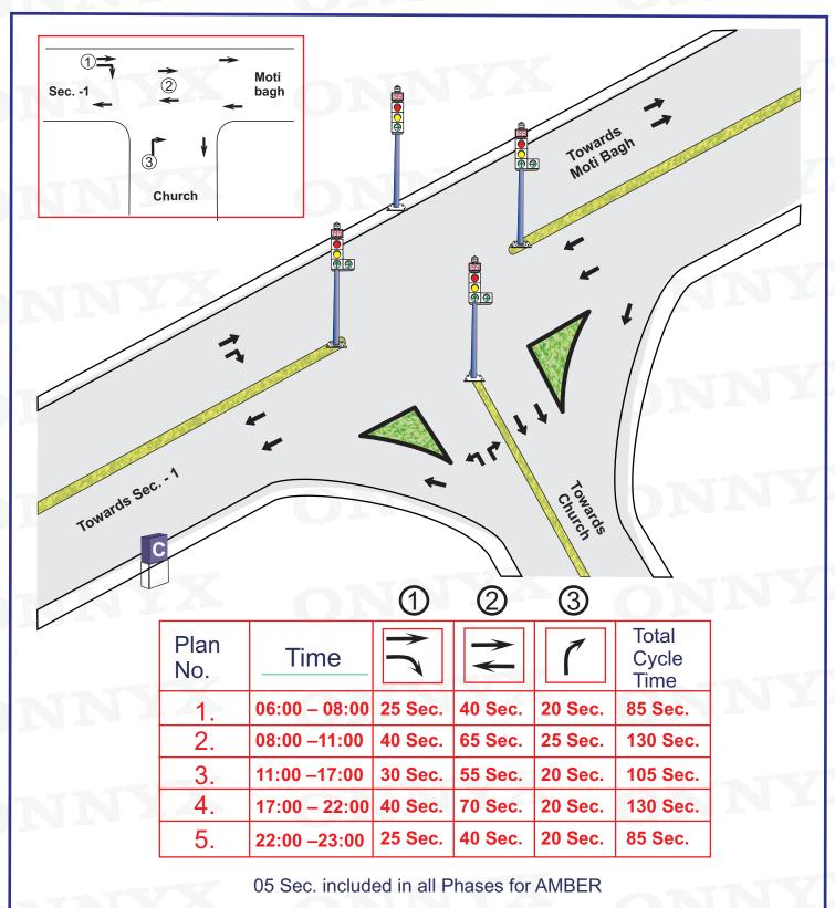
Signal Timing – 06:00 – 23:00 Blinker Timing – 23:00-06:00
