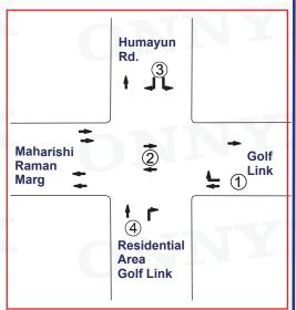
Signal Timing - 06:00 - 23:00 Blinker Timing - 23:00 - 06:00
